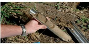
carefully, using the slip wrench if necessary. Carefully open the split cup set to examine the sample. If a liner was used cap the ends with the provided end caps.
