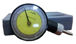
**DESCRIPTION:** Geotester dial penetrometer set is used for on-site measurement of soil compaction by testing the foundation plane or boring samples. It gives readings of estimated unconfined compressive strength in TSF or kg/cm2 when used with the standard 1/4" dia plunger. The geotester is furnished with stainless steel plungers, carrying case, data tables, register plates and instructions.
