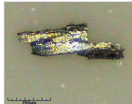
Metal particle from screw thread
