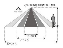
This sensor detects changes in infrared radiation that occur when a person (or object) moves whose temperature is different from the environment.
