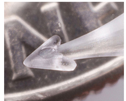
Bioresorbable tissue anchor with better than .0045" radius on end of barb
