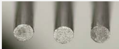
.018” 45 degree view of wire bond end. Perfectly formed, flat, evenly finished, sharp edges are ideal for bonding
