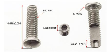
A domestic manufacturer of aerospace latching systems approached MW Components to develop a custom CRES fastener for a new product design in an airframe latch. The part's design involved three different geometric challenges: a convex head feature, a reverse hex extrusion, and a rolled thread over the backward extrusion.
