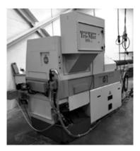
Star and Citizen CNC equipment capable of producing highly precise complex parts. Diameter capacity up to .750". Tolerances can be held to +/- .0002".
