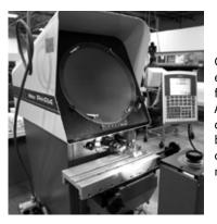
Optical Comparator inspection equipment for in-process and first article measurements. Also a key tool in the detection and prevention of burrs, scratches, indentations or any other imperfections in material or finished product.
