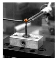
The zone annealing process passes a heating zone over a specific area that generates a sharp gradient in a part. This enables the adjustment to the shape of the part in raw form.
