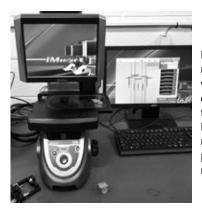
IM-6225 Keyence instant measurement system. A visual inspection system that drastically reduces inspection time and operator subjectivity. Enables us to measure multiple parts at one time and provide that information in a report.
