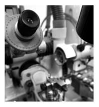
Precision microscope further enhances the inspection process for the smallest diameter products. It gives us the ability to measure against X, Y, and Z axis at high magnification and detect the slightest variance.
