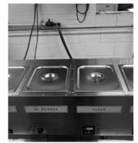
Heated ultrasonic filtered cleaning system with de-ionized water filtration. Ensuring the removal of trace amounts of contaminants and particles prior to the addition of precious metals plating.
