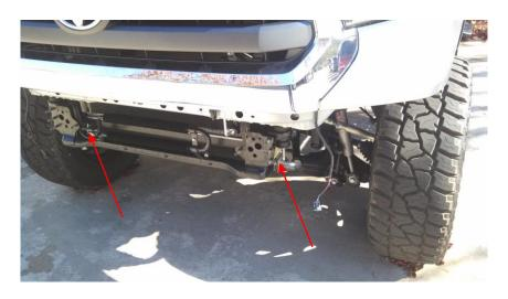
**Figure 3 - Factory Bumper Connection**
