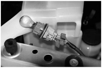
**Figure 12 - Turn Signal Wiring Access**
