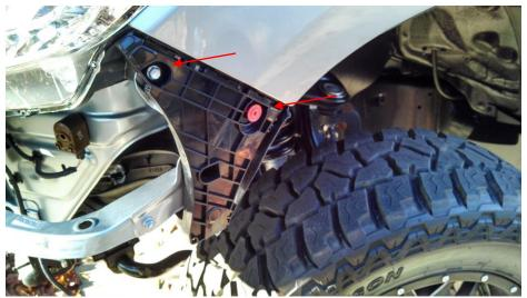
**Figure 7 - Spacer Fastener Locations**
