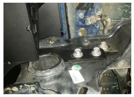
J. Align the bumper top to bottom to ensure a perfect fit to the truck. Allow for a 0.375" clearance to all painted surfaces if possible to allow for frame flex.
