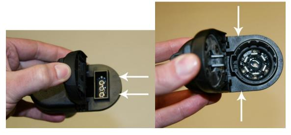
C. Install the trailer plug into the cutout in the new bumper using the #8 hardware supplied.
