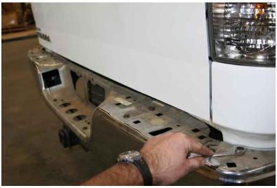
G. Remove the OEM bumper and set aside. Hold onto the
