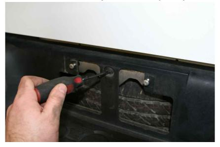
E. Pop the plastic clips loose on the bottom side of the main piece of plastic on the top side of the bumper allowing access to the OEM fasteners.
