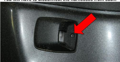
Figure 1 – License plate light removal
