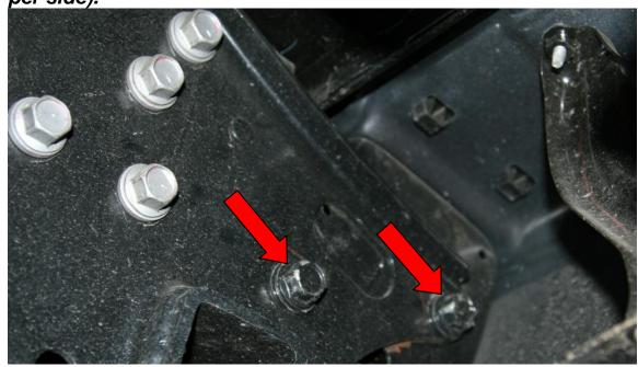
Figure 4 – OEM bumper bolt removal
