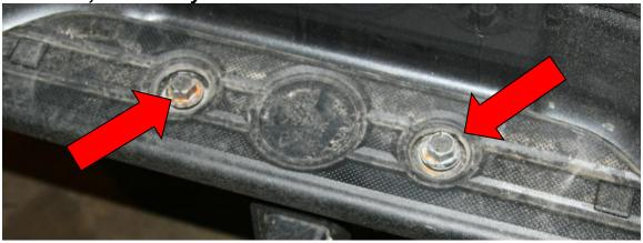
Figure 3 – Trailer hitch bolt removal
