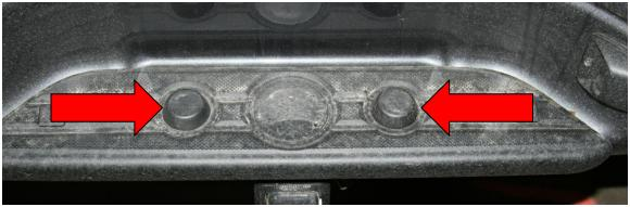
Figure 2 – Bolt cover removal
