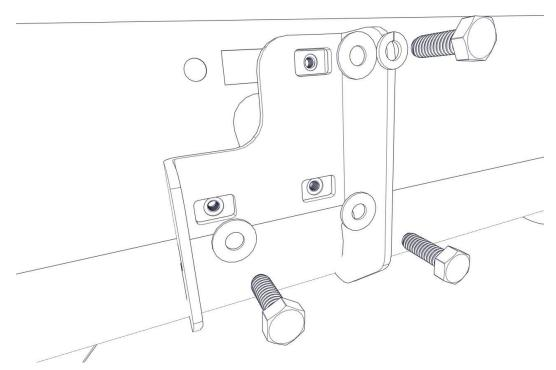
Figure 7 - HARDWARE STACKUP FOR MOUNTING SIDE STEP
