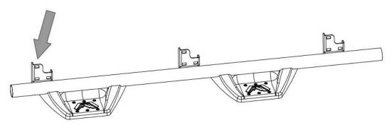
Figure 5 - ADD FRONT 5/16-18 BOLT TO HOLD STEP FIRST
