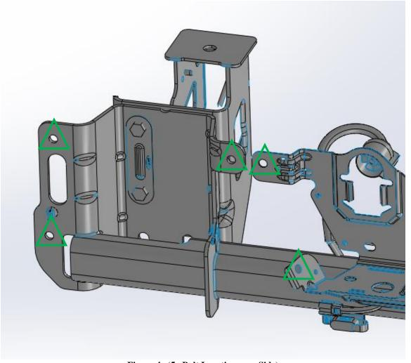
Figure 4c (5x Bolt Locations per Side)
