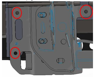
Figure 4 (3x per side, Outer Bolt Locations)
