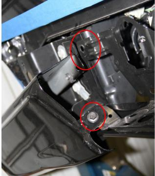
Figure 4b (2x per side, Inner bolt locations)
