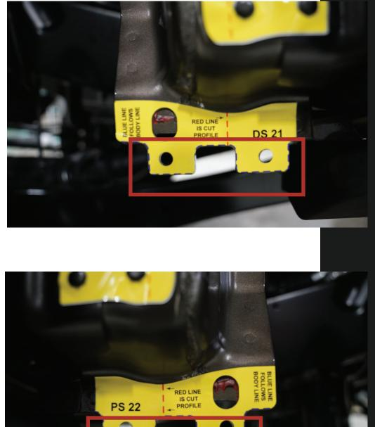
Bottom of cut template 21 on the driver side of the vehicle and the cut template 22 on the passenger side will be aligned with the profile of the bottom of the rocker panel indicated by the red squares.
