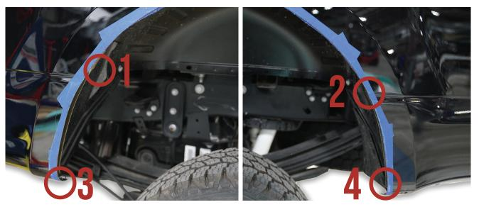
Using a chalk line, mark the cut line from the point where the indent in the rear fenders meet the wheel well cuts (ref 1 &2) to the bottom of the quarter panels before the wheel well structure meets the bed (ref 3 & 4).
