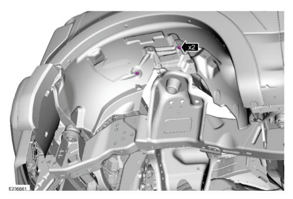
Using a plastic pin remover, T30 torx head and an 8mm socket, remove all the clips and screw indicated in the images above. If you do not see retainers for wiring harness in step 4 pull away liner from vehicle.
