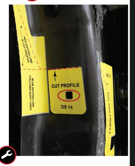
Cut template 14 will be aligned with the square cut in rocker panel, indicated by the red oval. This is the second square from the bottom of rocker panel and you may need to remove a black plug to see it. The first square maybe covered by tape.
