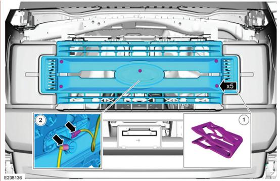
There are numerous locating clips holding the grille to the vehicle. Referring to the images above, slowly and firmly pull away the grille near the pink spotted locations. If you have the option for the 360 camera, disconnect the camera washer hose and the electrical connector (i.e. sub image 2) before pulling grille away from vehicle.
