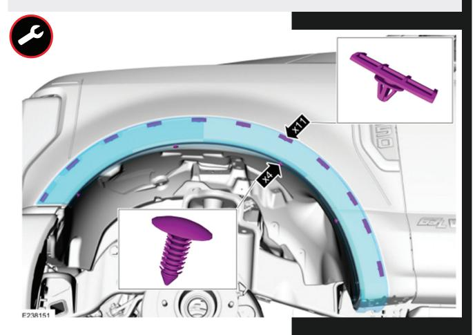
Using a plastic pin remover and a non-marring trim tool, remove the 4 pin and disengage the 11 retainers from fender.
