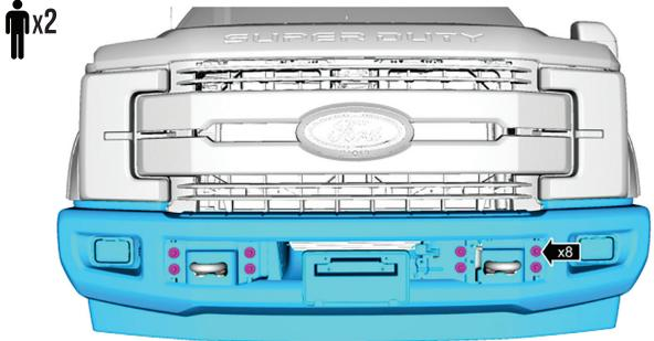
With the help of others, and using an 18mm socket, remove the 8 bolts holding the bumper to the vehicle. Pull bumper away from vehicle.
