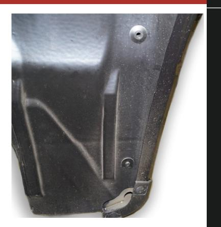
Using a plastic pin remover and a 7mm socket remove the 3 bolts and 3 pins holding the inner and pull the inner lining away. There will be a bolt and pin combination on the front, back, and inner faces of the wheel well liner.
