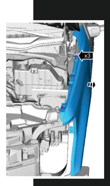
Using a box cutter or its equivalent, cut away the foam baffle along the body. Locate the 3 bolts at the top of the fender toward the engine bay and using a 10mm socket remove them. With the help of another you can now pull the fender away from the vehicle.
