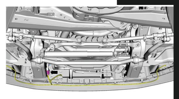
Using a 5.5mm socket remove and the plastic fastener remover, remove the 2 bolts and 2 Christmas tree pins holding the filler plates from both sides of the vehicle. Using a 15mm socket disconnect the 2 extension bolts from both sides of the vehicle. Finally, disconnect the electrical harness at the indicated location above.
