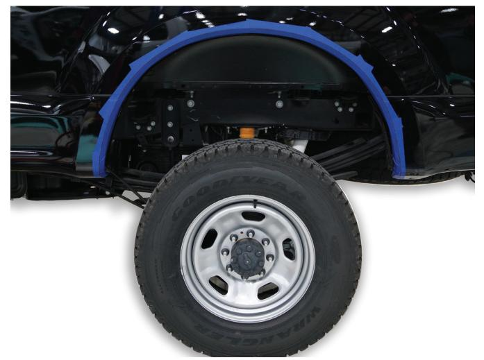
The rear fenders of the vehicle will be covered with painters tape along the contour shown beside. At this point the contour will be marked to indicate the cutting line.. Using a cutoff wheel, the indicated portion of the fender will be removed.
