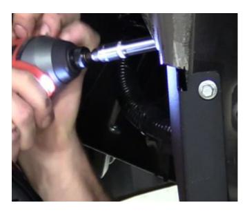
Using a 5/32" bit, drill pilot holes. Reinstall plate on vehicle, using a 3/8" socket and provided self-tapping bolts. With plate installed, tape around edges leaving a gap at the top for the provided foam tube to fit
