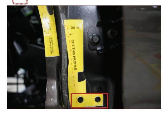
Bottom of cut template 11 will be aligned with the two bolts in side of rocker panels, under door hinges, refer to red square.
