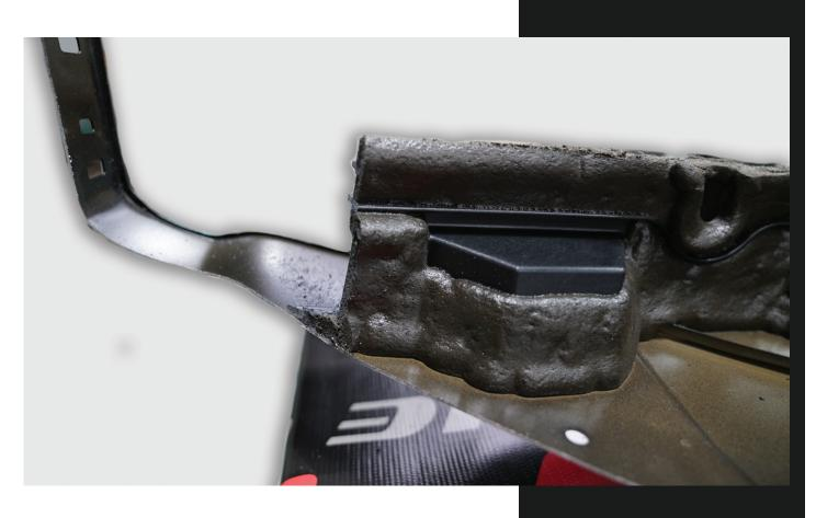
Using a body saw, flip the fender over and cut off the plastic mold along initial cut line.
