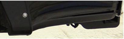
Using shears, cut off the front portion of the kick panels. There should be enough material left to tuck under fender flange. Reinstall kick panels inserting front under fender flange (ref. oval) and using pins to clipping in rest (ref. arrows).
