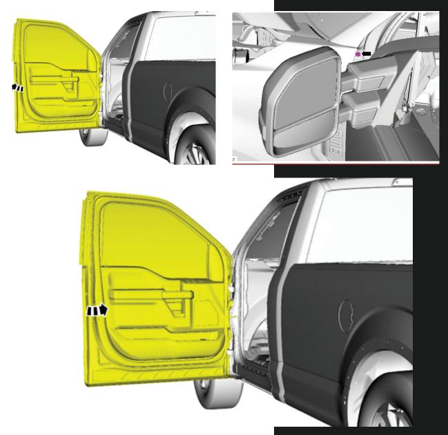
Open the door to gain access to the bolt located in the door jamb toward the top of the fender. Using a 7mm socket remove the bolt. The bolt may have been powdered over making it difficult to grip with the aforementioned socket. Once the bolt is removed close the door.
