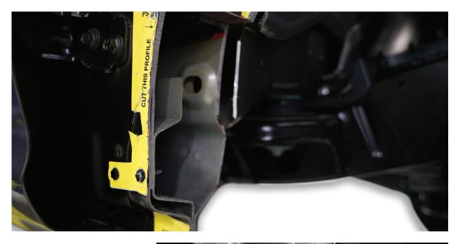
Take care when cutting template 6 cut line. Do not over cut and penetrate the firewall.
