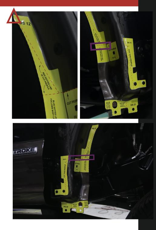
Start at the top of cut template 12 by matching the contour of the template to the vehicle indicated by red triangle. The red dashed lines of the cut profile should align with the cut template 14.
