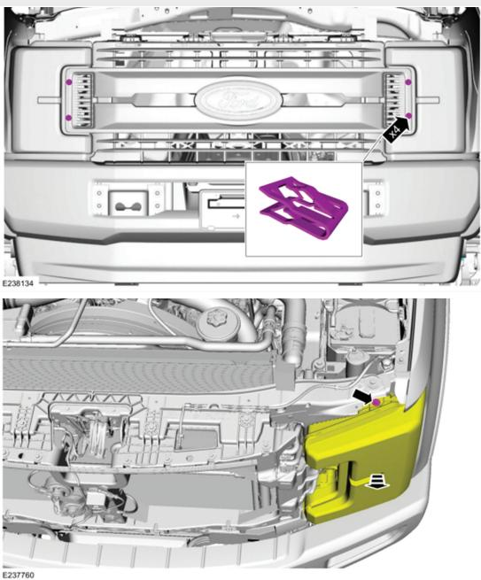
Using a 10mm socket remove the 4 retaining bolts securing the inner corner, bottom outer corner, and top of headlight where indicated in the images above. Slowly pull away headlight from vehicle until electrical connector can be seen.
