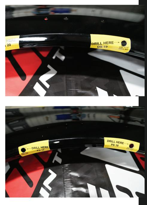
With cutting templates installed you can now drill. Using a center punch and 17/32 bit, mark and drill holes at the locations indicated by the templates.
