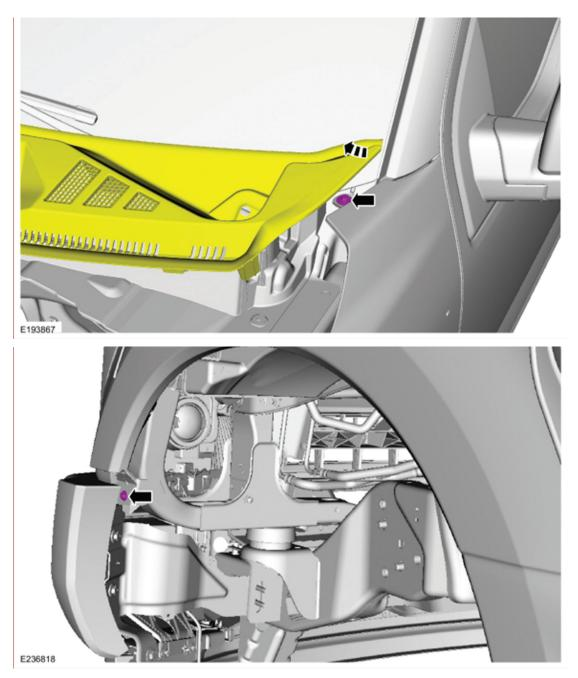
Raise the corner of the cowl to access the bolt underneath, then using a 10mm socket remove bolt. Now, locating the bolt at the front lower mount of the fender use a 10mm socket to remove.
