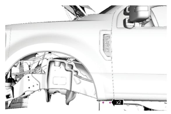
Using a 10mm socket remove the 4 retaining bolts securing the inner corner, First locate the fender insulator on the inside of the wheel well and slowly pull away from vehicle. Using a 10mm socket remove the first 3 bolts securing the fender to the cab.
