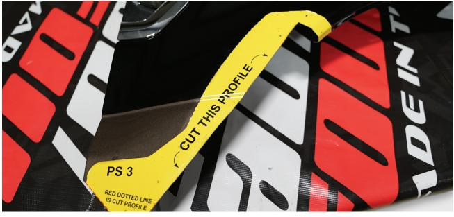
The last step in the front fender cut is to return to cut templates 3 & 1 and to cut off the bottom portion indicted by the red squares. This will remove the rear most bottom of the fender.
