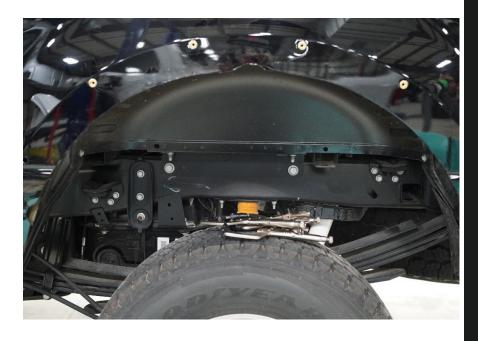
Once fender fits flush to the vehicle clamp fender in place at top and bottom flanges. Use a 25/64" center punch to punch all holes.
