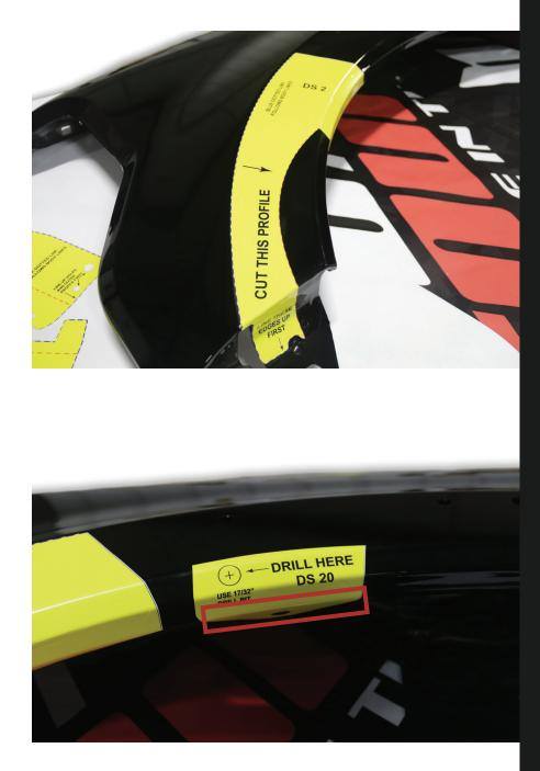
Start by installing cut template 2 on the front bottom edge of the fender of the vehicle. Cut template 2 will be installed by aligning the bottom edge profile with the matching sheet metal of the fender indicated by the red oval. When placing the template, make certain the template is aligned with the contour of the fender, ref purple crescent. Cut template 4 is a mirror of cut template 2
