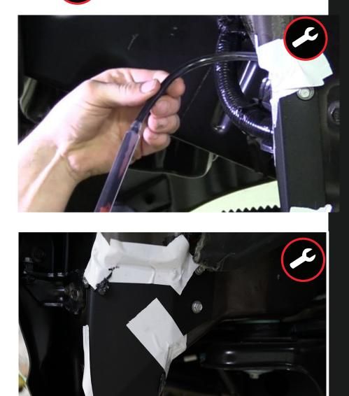
Using foam sealant fill in all gaps, then cover areas of application with duct tape and leave to set. After dry remove duct tape, remove excess. Note: read the directions and warning labels on provided sealing foam for instructions on proper application and use.
