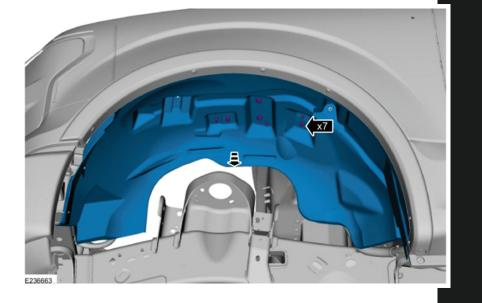
Disengage the 7 retainers for the wiring harness at top of inner fender and pull away from vehicle.
