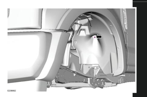
Remove single screw in middle rear of inner fender.
