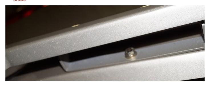
Install seal around edge of fender flare. Using a 1/2" socket/ratcheting wrench, Install fender flare. Install all bolts hand tight. Surrounding images show bolt installation. Leave bolts extremely loose until all bolts have been installed.
