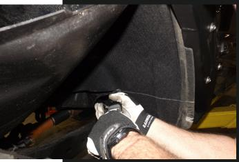
With Felt inner fender installed cut plastic covering to match felt in the back with a larger cut in front.
