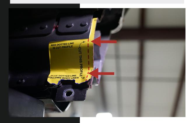
Any cut not in line with red cut line should be ground or cut back to match for proper fitment of accessories. The above cut is a good example of leaving too much material.
