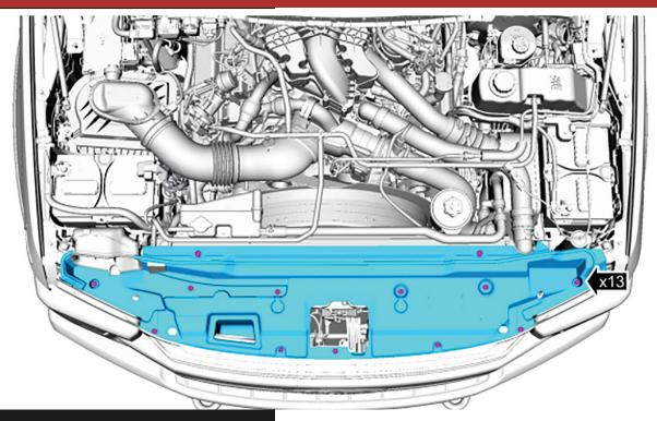
Using a plastic fastener remover, remove the 13 push pins from the radiator cover and 1 pin from the intake, then lift radiator cover from engine compartment.
