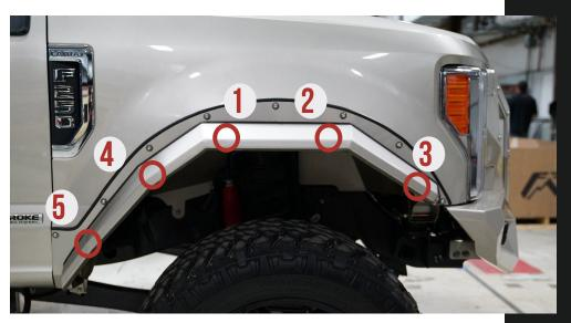
Using a 1/2" socket/ ratcheting wrench, Install fender flare. Install all bolts hand tight.
