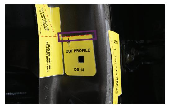
Top of cut template 11 will be aligned with the cut profile of cut 14, refer to purple square.
