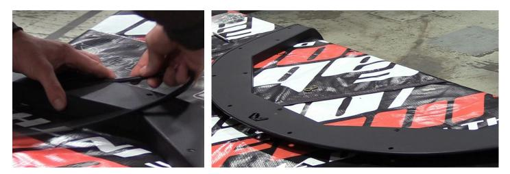
Run seal along outer edge of base, cutting the excess off after full installation. With seal installed used the provided stainless steel hardware and nut plates to install fender base.
