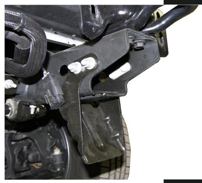
With the bumper off the vehicle, you can now remove the tow hooks by removing the four 18mm bolts located under the top of frame rail. Next, using 18mm socket remove the two nuts on either side of the frame attaching frame horns to frame. Set bolt strips and nuts aside as they will be used in the installation of Fab Fours bumper. Repeat on other side of vehicle.
