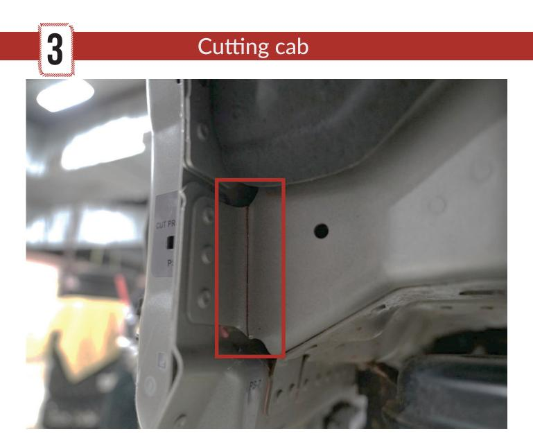
Using a sawzall cut through the radius of the flange indicated by the red square on above.
