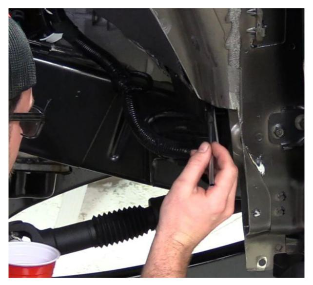
Using an acid brush apply a coat of 'Rust Trap' to ALL cut edges and exposed surfaces to prevent corrosion. Above is an example of application in the cab cut area.
