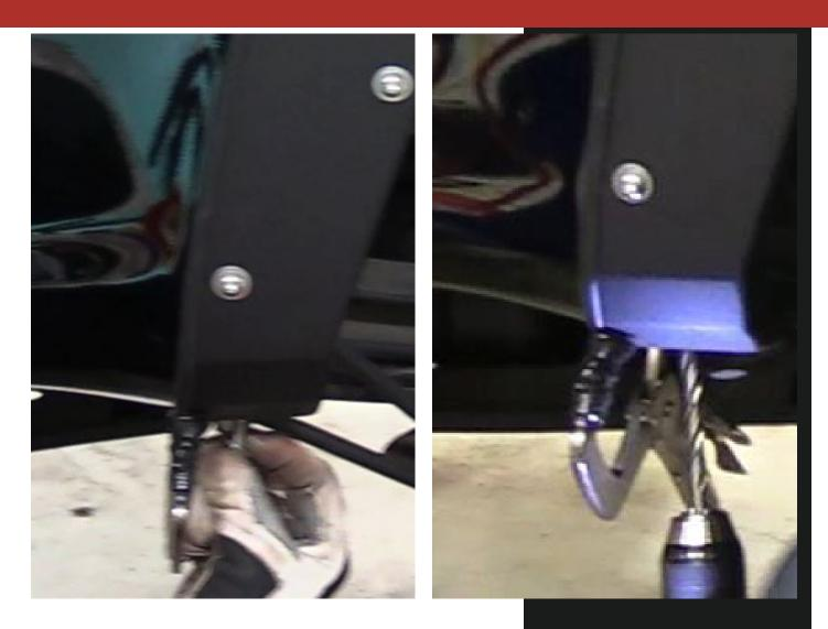
With the stainless steel hardware fully bolted, drill clearance holes for 5/16" zinc bolts at the slots located at the bottom corner on each side.
