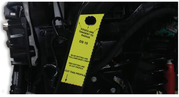
Cut template 15 and 9 are installed by placing all edges on the flat of the tube where the different curves end. This is done by attempting to align the slot and lineup edges of the templates on both sides with the flat part of the tube, right before it starts to curve.
