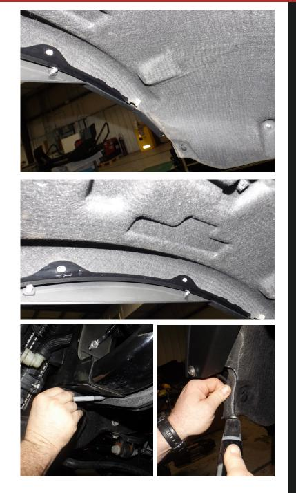
The front OEM inner fenders can be reused with a little modification. Using a small reciprocating saw the plastic/felt can be cut. The profile of the cut is a suggestion and can be modified based upon the opinion of the installer/customer.
