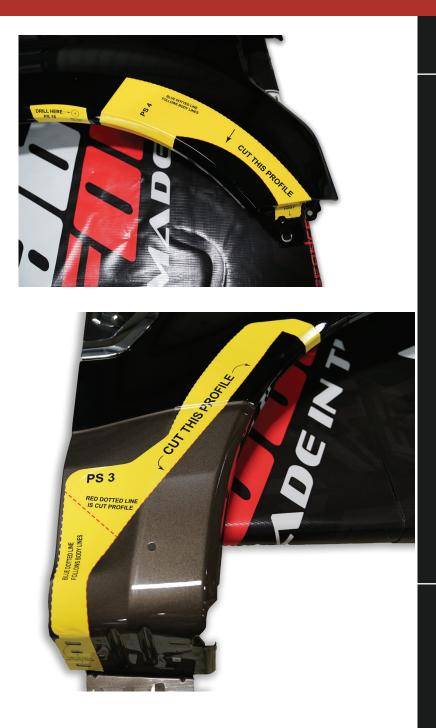
Cut template 4 is the passenger side template and a mirror of the driver side. Repeat steps for Cut template 2
