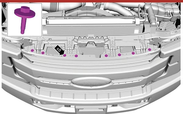
Using a 10mm socket remove the 8 bolts indicated in the image above.
