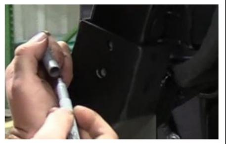
Insert lower portion of reinforcement bracket into cut, making sure the top of the brace is flush with the top mounting surface of the bracket. Hold the bracket to the reinforcement brace as shown besides. Mark the drill locations using a marker, a center punch, and the bracket hole as a guide. Use a 1/4" drill bit for a pilot hole. Do this on both sides of vehicle.
