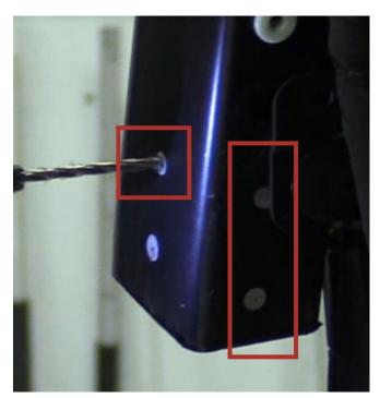
Using the provided drill bit for rivet, drill the top three holes indicated by the red squares in the image to the right and follow the rivet nut instructions1 to install the three rivet nuts in the reinforcement bar.
