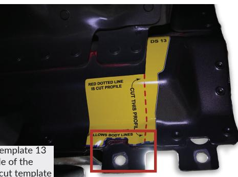
Bottom of cut template 13 on the driver side of the vehicle and the cut template 7 on the passenger side will be aligned with the inside profile of the bottom of the rocker panel indicated by the red squares.
