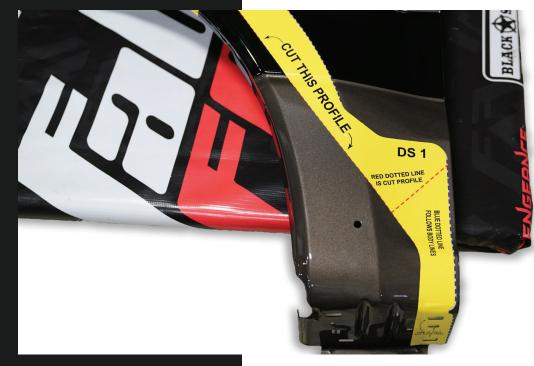
Cut template 1 will be aligned with the holes on the bottom of the fender and the outside contour of the fender. These two areas are indicated by the red ovals in the images around the box. Cut template 1 is the driver side template and a mirror of Cut template 3.
