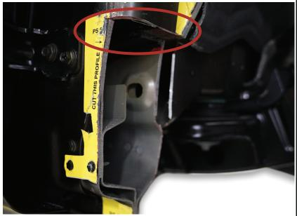
Next cut lower rocker channel away, starting from the bottom of the cut template 22 and up through cut template 5. This cut will pass complete through rocker panel not following cut template 7, refer to the image to the left.
