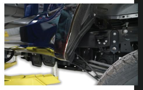
Using saw the final cuts should look similar to photos here on both sides of truck.
