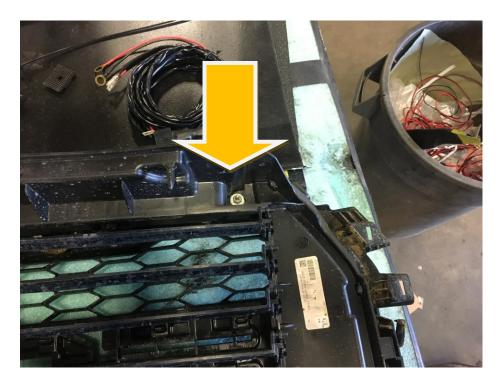
B. Using 10mm socket, remove stamped nuts at the bottom of the grille.
