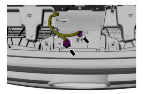
C. Note for vehicles equipped with fender mouldings: Remove the 2 screws and release the 3 front fender moulding retainers and position the fender moulding out.
