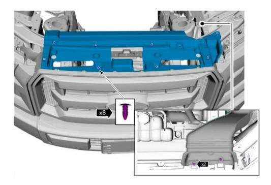
**B.** NOTE: As truck is equipped, disconnect the electrical connectors and washer hose.
