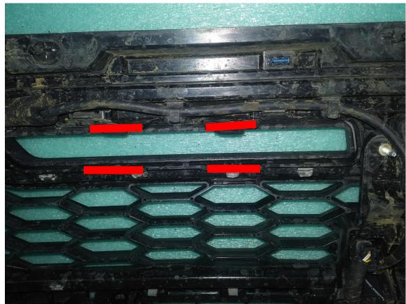
E. Position radar bracket on louver frame and mark holes 7/8" from center of louvers. Keeping back tangent with lip of frame.
