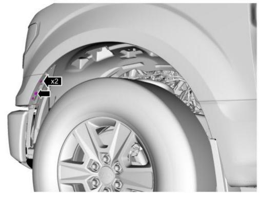
E. Remove the pin-type retainer.
