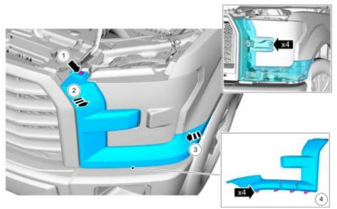
G. Remove the air deflector from the grille on both sides.
