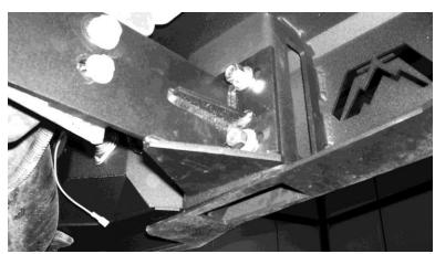
**B**) Bolt bumper to mounts using supplied hardware as shown in Parts List.
