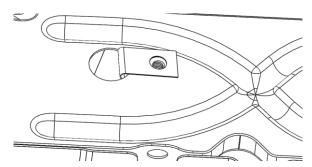
Figure 5 - ADDING M8 NUT CLIPS FOR REAR SIDE STEP BRACKETS
