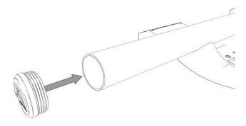
Figure 4 - INSTALLING THE FABFOURS SIDE STEP END CAPS
