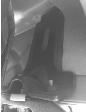
Figure 3 - OEM CHEVY HD UPPER SUPPORT BRACKET
