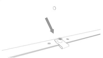
Figure 6 - FRONT M8 NUT CLIP INSTALLED ON PINCH SEAM
