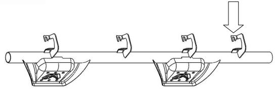
Figure 6 – ADD REAR M8 BOLT TO HOLD STEP SECOND
