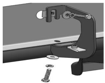
Figure 7 - BOLTS INSTALLED THROUGH THESE BRACKET HOLES
