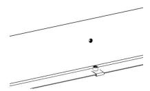
Figure 3 - ADDING M8 NUT CLIPS FOR REAR SIDE STEP BRACKETS
