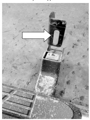
Figure 1 - OEM CHEVY/GMC SIDE STEP MOUNTING BRACKET
