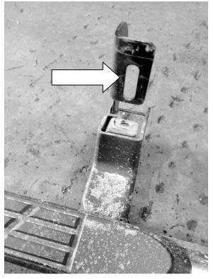
Figure 1 – OEM CHEVY/GMC SIDE STEP MOUNTING BRACKET
