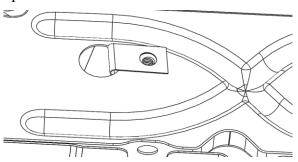
Figure 3 - ADDING M8 NUT CLIPS FOR REAR SIDE STEP BRACKETS
