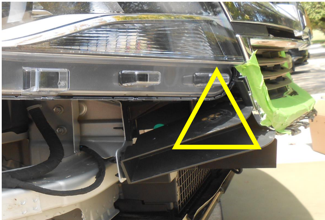
Figure 5d (mount point on plastic grill mount)
