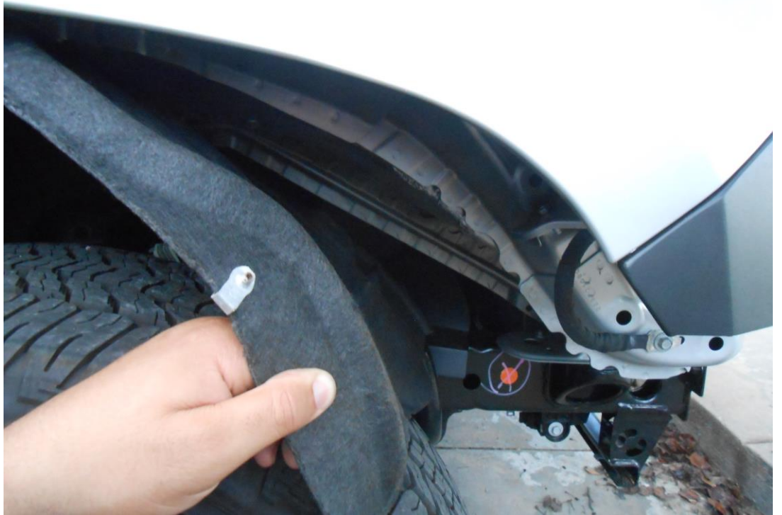
Figure 6a (wheel well liner pull back)
