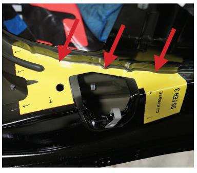
Cut Template DS FEN 3 is placed on the backside of the driver's side front fender. Start applying the template by lining up the profile shown with the red arrows. Then work the template across matching the locating hole with the one on the fender.
