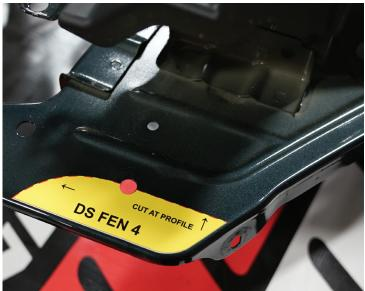
Cut Template DS FEN 4 is applied to the front side of the driver's side front fender ahead of the fender well opening. Align the edge of the template with the fender profile and the locating hole as shown.
