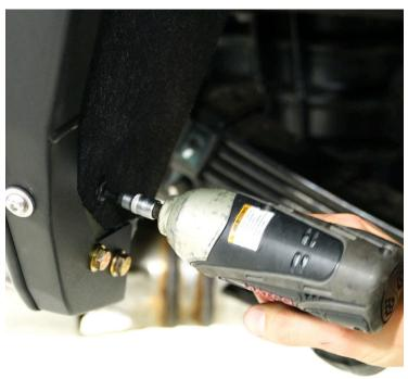
To reinstall the OEM inner fenders, they will need to be trimmed.
