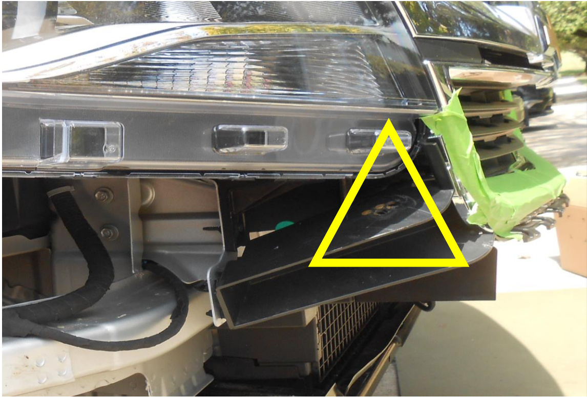
Figure 5d (mount point on plastic grill mount)
