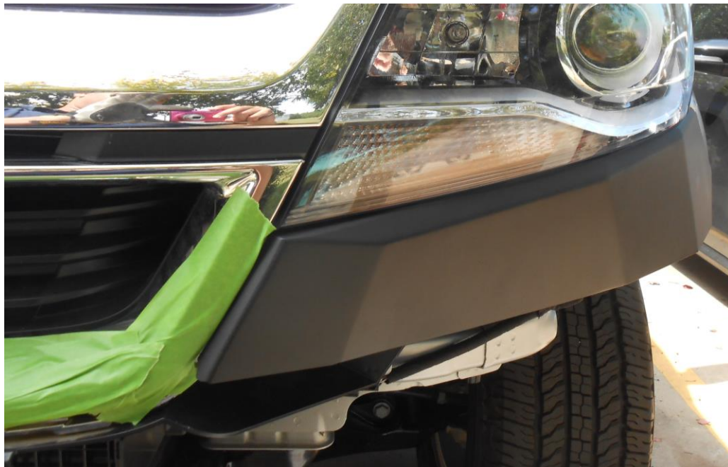
Figure 5c (valence position relative to grill)
