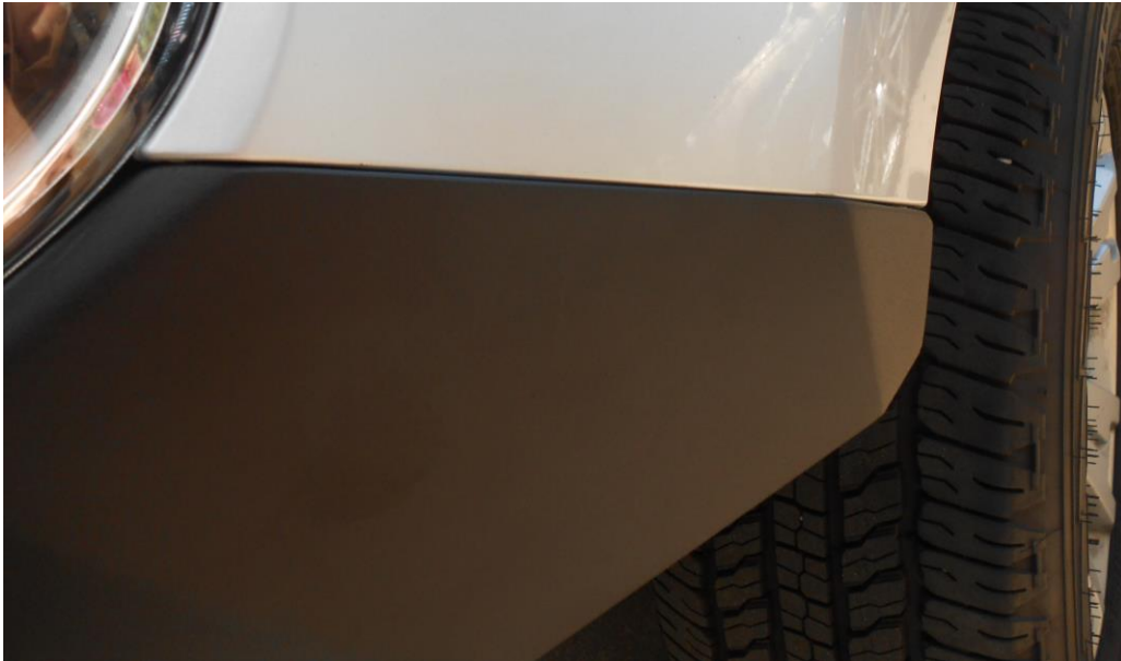
Figure 5b (valence position relative to fender)
