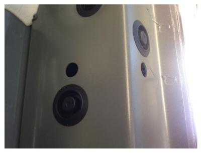
3) Once plugs are removed install M8 nut clips as shown below.
