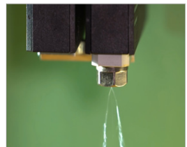
Perfect interaction of spray air and adhesive
