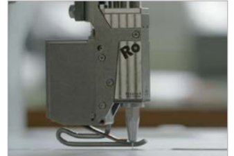
Cold Glue Application
