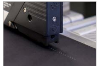
Hot Melt Dot and Bead Application
