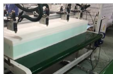
Spray application on foam
