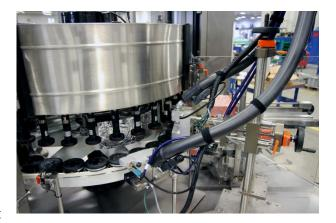
at affixing pre-cut paper or film wrap-around labels to cans, bottles, or jars of widely differing sizes and shapes. Canmatic uses minimal glue to accomplish this because the label is held in place by just two narrow lines of dispensed hot melt glue.
