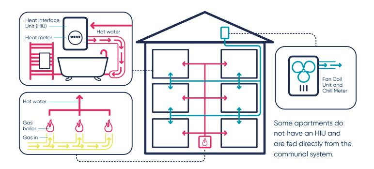
Rather than have an individual gas boiler in every home, a communal heating system uses a centralised boiler to provide heat for the whole development.
