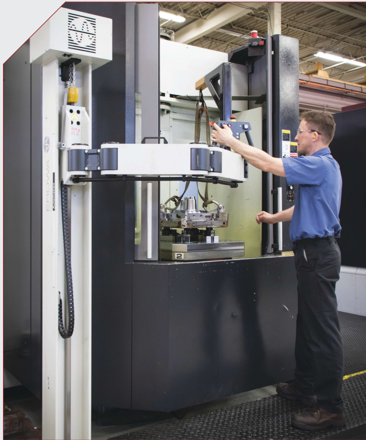
This Erowa Lift system has proven far easier on employees who had gotten used to lifting heavy pallets onto a crane. It's also saved time by eliminating the need to share a crane with other workstations.
