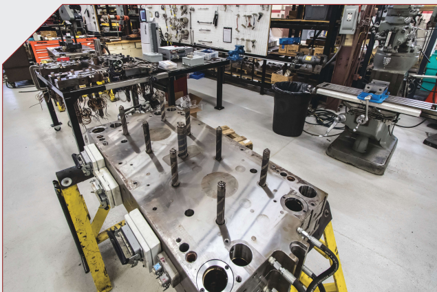
Departmentalizing the shop has long helped facilitate attention to detail in metal-cutting operations. Now, Ai Tool is seeking to realize the same advantage elsewhere by departmentalizing other functions of the mold build as well. This station, for example, is dedicated solely to assembling and wiring hot runner systems.
