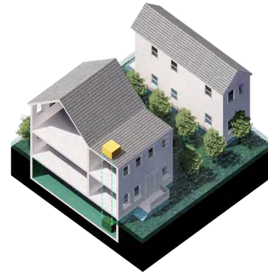
RAISING CRITICAL SYSTEMS
