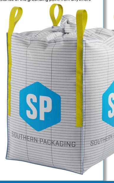
Bag made of woven fabric which enables electrostatic charge to be dissipated without being grounded. The fabric of a Type D FIBC generally contains conductive threads or filaments which safely dissipate the charge through low energy "corona" discharges. Some Type D bags have a low resistivity lining, which can reduce the risk of incendiary discharges. Type D bulk bags are safe for transporting FLAMMABLE products. Flammable materials or gases MAY be present outside of the bag.
