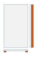
Display board showing addition of side studding to provide hollow back.
