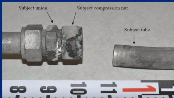
▲ A loose section of tubing connection from a sulfuric acid sample station responsible for the release of 84,000 pounds of sulfuric acid into the environment.<sup>4</sup>
