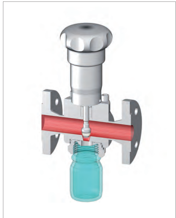
Principle of conical seat
