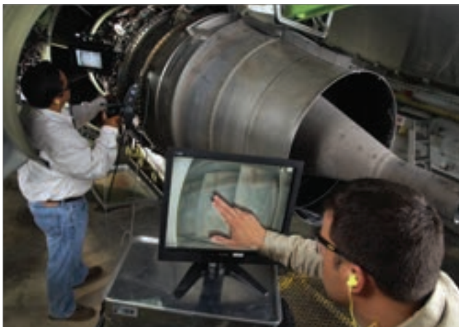
The same inspected image is shared between two operators with an external display connected to the IPLEX RX for remote observation
