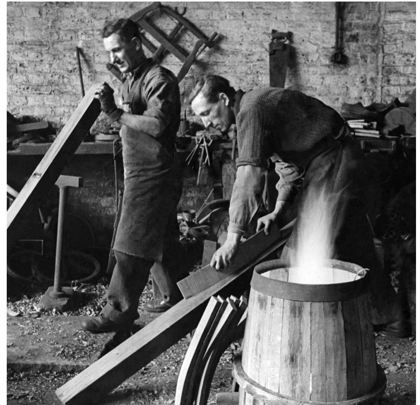
ABOVE: Making navy casks. Albert Pearcey a cooper of Rotherhithe, whose father and grandfather practised the craft is busy converting big wine casks into handy containers. April 1944 Rotherhithe.
