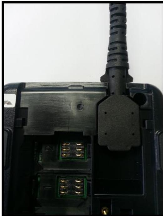
3. Replace the back plate and tighten the screw. (*See image below*)
