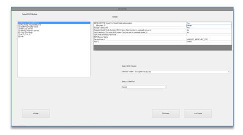
Select the Verifone VX805 – Encrypted No sig cap option and select the com port you assigned the VX805 to in the step above.
