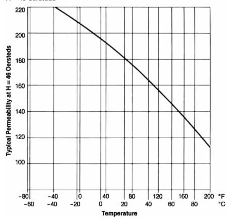
Typical Temperature-Permeability Curves Carpenter Temperature Compensator "32" (Type 1) at various magnetizing forces below 46 oersteds
