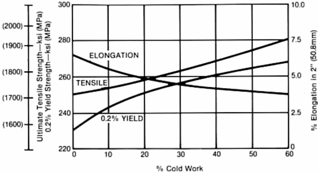
**Effect of Cold Work on Typical Tensile Properties of Custom 455 Stainless Wire**
