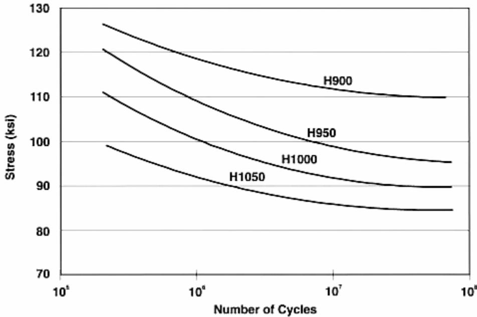
Typical Constant Life Fatigue Diagram for Custom 455 Stainless Bar in the H 1000 Condition at Room Temperature
