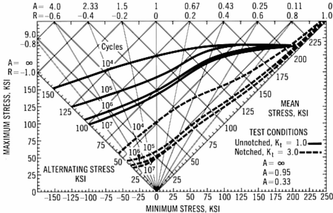
**Typical Constant Life Fatigue Diagram for Custom 455 Stainless Bar in the H 950 Condition at Room Temperature**
