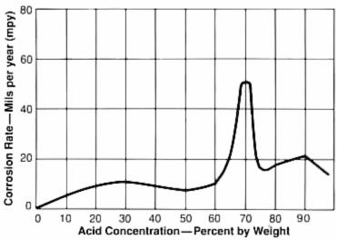
Typical Iso-corrosion Properties in Sulfuric Acid - 20Cb-3 Stainless
