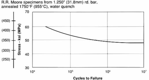
Typical Room Temperature Mechanical Properties - 20Cb-3 Stainless Annealed 1750°F (955°C), water quenched
