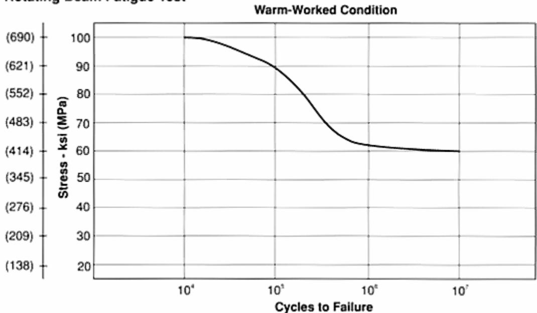
Typical Room Temperature Mechanical Properties - 15-15LC Modified Stainless
