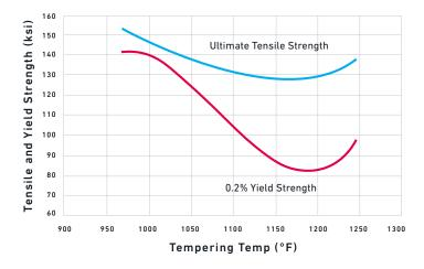
Hardened  $1800^{\circ}F$  (982°C) 1 hour, oil quench, tempered 8 hours.
