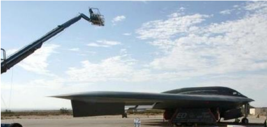
ARAMIS Thermography being done on B2 bomber
