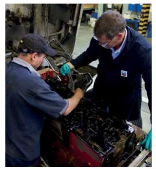
The final inspection overall showed a clean engine with minimal deposits and wear on the key engine components. The pistons showed minimal deposit build-up on the crown and top ring land zone. The camshaft lobes showed excellent wear protection and no visible wear scars on rollers or rocker arms.
