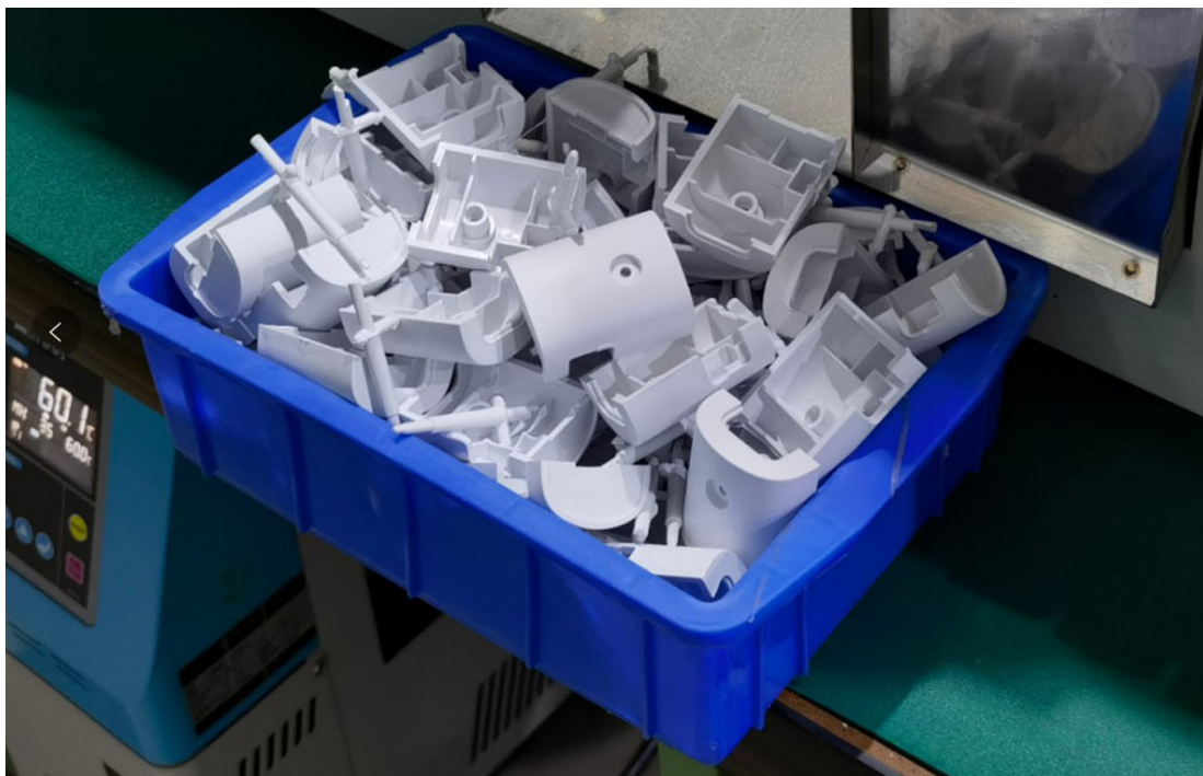
Freshly injection-molded ABS control box housings using the Rigid 10K molds.
