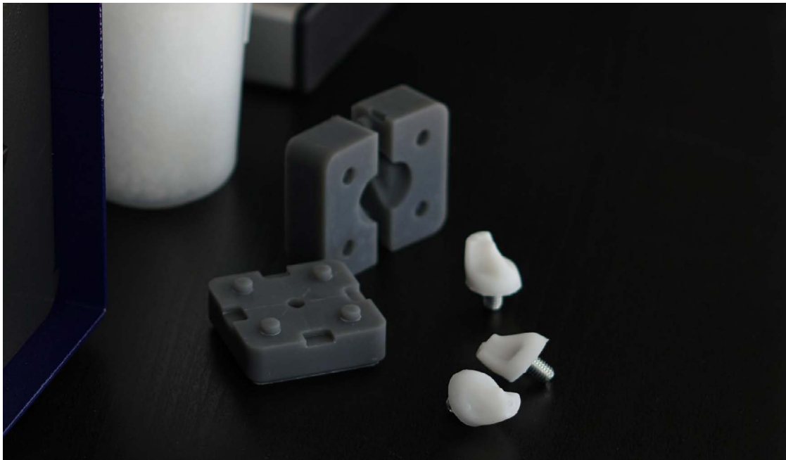
POM football cleats injected in the Holipress from molds printed with Grey Pro Resin.
