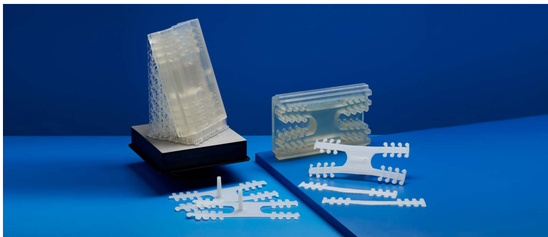
The mold printed with High Temp Resin next to the two-strap injected in polypropylene
