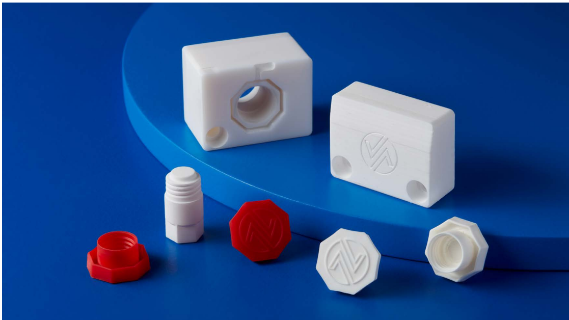
The printed three-part mold with the caps injected in polyethylene.
