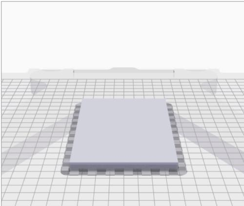
The Raised Part feature prints the part above a thin layer of supports. Turn on for the most consistent surface resistance.
