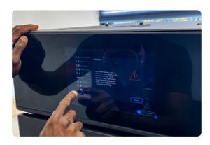
5. Start the print: Once all preprint checks have been completed, the Fuse 1 is ready to print. The home screen transitions to display a live stream of the print bed so you can watch each new layer take shape. This camera view is also available in PreForm.
