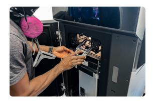
3. Insert a build chamber: Carry the build chamber between the Fuse 1 and Fuse Sift using its integrated handles, no casters or support frames necessary. Having multiple build chambers in your workflow enables you to run another print while a previous one is still cooling.
