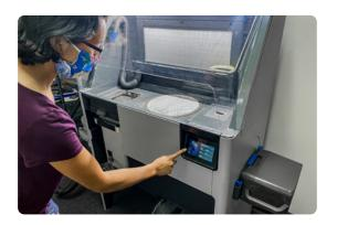
2. Start the sifter: As parts are extracted from the cake, unsintered powder is dislodged and funneled into the sifter below the workspace. A sieve filters out any small chunks or debris to keep the powder clean. The reclaimed powder is then stored in a dedicated hopper until mixing with fresh powder for the next print.
