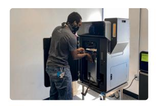
4. Preprint checks: A checklist on the touchscreen with written and visual instructions explains each procedure step by step. The Fuse 1 monitors itself over time, and automatically notifies you when a maintenance procedure is required.
